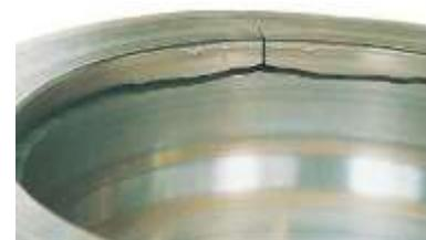
Fig. 3: Bearing crack
