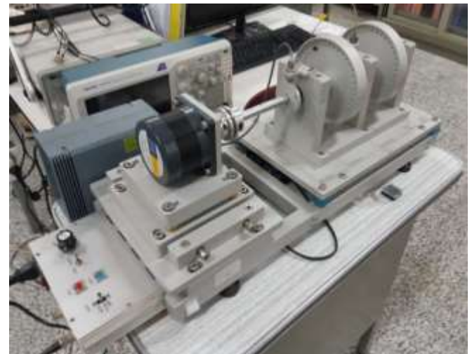
Fig. 3: Rotating Motor Test Bed for Bearing Data
